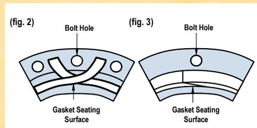
3. Overlap the ends of the sealant to complete the seal (fig. 2). On fragile flanges with low clamping forces, use an angled cut joint 1-2 times the seal's width (fig. 3).
