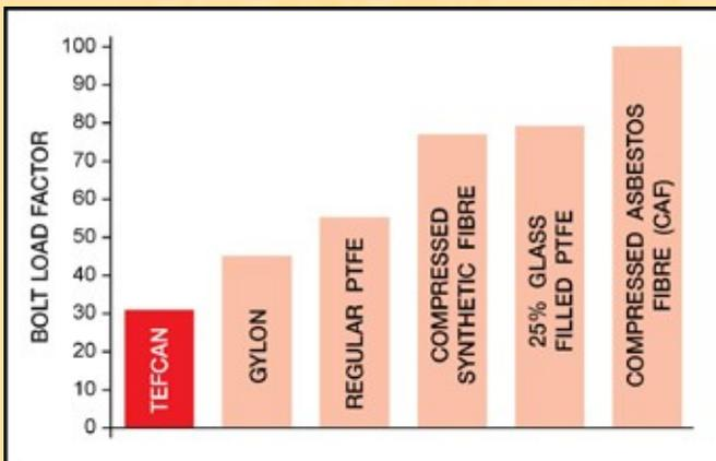
Tefcan requires less than 1/3 of bolt load required by CAF to seal when tested at 30 psi gas on a rough surface flange.
