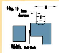
2. For rough surfaces, select a size with a nominal width (  $d$  ) that is approximately 1/2 of the gasket contact area (  $W$  ). On scored surfaces, overlap sealant at the location of the score, or lay in an extra piece to double-up the material.
