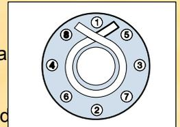
5. Very occasionally some spools may contain a splice covered with adhesive tape. If found, cut out the splice, and continue the gasket by overlapping the two ends for approximately 12 mm.
